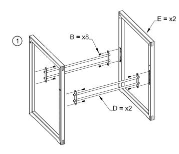
1. Secure the two stainless steel tubes assembly in place using the supplied allen key and 8pcs flat head bolt M6x16mm - Do not fully tighten the bolts, instead secure them loosely in place with two turns only
