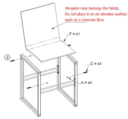
2a. Line the seat/back assembly up with the 4 upper holes in the teak frames and secure them loosely in place (two turns only) with the custom bolt M8x50mm - Note that there must be  $\emptyset$ 12x7mm spacers between the teak frames and the seat assembly
